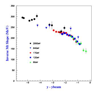
**Figure 3:** Inverse  $m_T$  slopes for  $k^-$  spectra from central AuAu and PbPb collisions versus  $y-y_{beam}$ for various energies. The data at  $\sqrt{s_{NN}} = 9,12,17$  GeV are from NA49 [15] while the BRAHMS results are from 64 (preliminary) and 200GeV [1].
