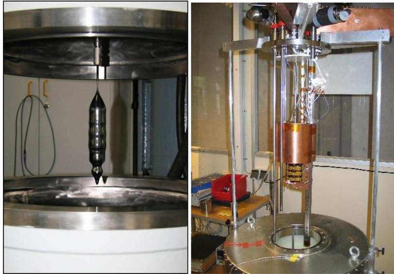
**Figure 3:** Left: Germanium crystal pulled with the dedicated Czochralski puller at IKZ, Berlin. Right: 18-fold segmented HPGe detector in the test stand. The detector was operated directly in liquid nitrogen.
