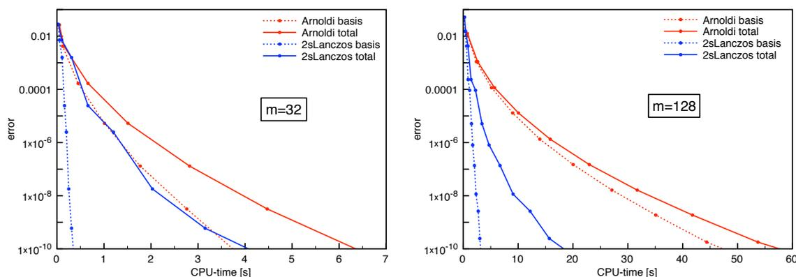
**Figure 2:** Accuracy versus CPU-time (in seconds), on an Intel Core 2 Duo 2.33GHz workstation, for the Arnoldi (red) and the two-sided Lanczos method (blue) for a  $4^4$  (left) and  $6^4$  (right) lattice.
