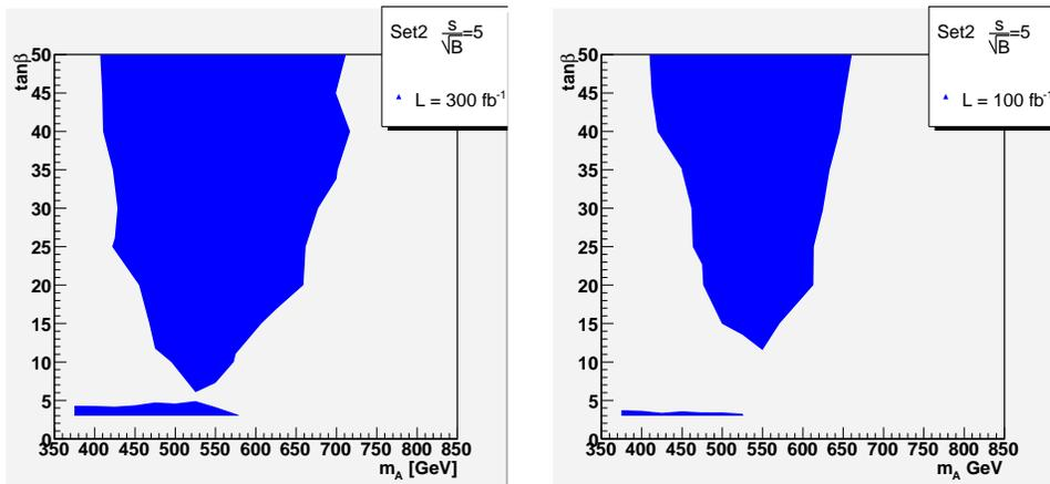
**Figure 3:** Discovery potential (for MSSM Set2) for Higgs boson  $A/H$  and  $H^\pm$  of mass  $m_A$  for final states with four leptons and missing transverse energy, as a function of  $m_A$ : contours are drawn for a search significance  $\frac{S}{\sqrt{B}} = 5$  for an integrated luminosity of  $\int \mathcal{L} dt = 300$  (left) and  $100 \text{ fb}^{-1}$  (right).
