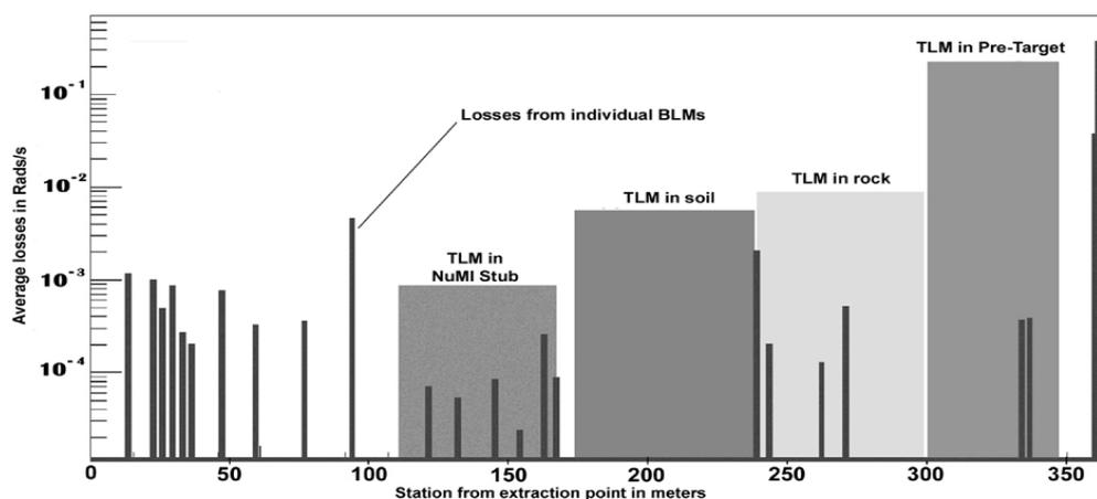
Figure 1. Beam loss along the NuMI proton line averaging for all beam extractions over a one month period. The beam loss scale can be obtained by the reading of the most downstream BLM which sees beam loss from the target profile monitor. This monitor scatters  $10^{-5}$  of the beam passing through it.
