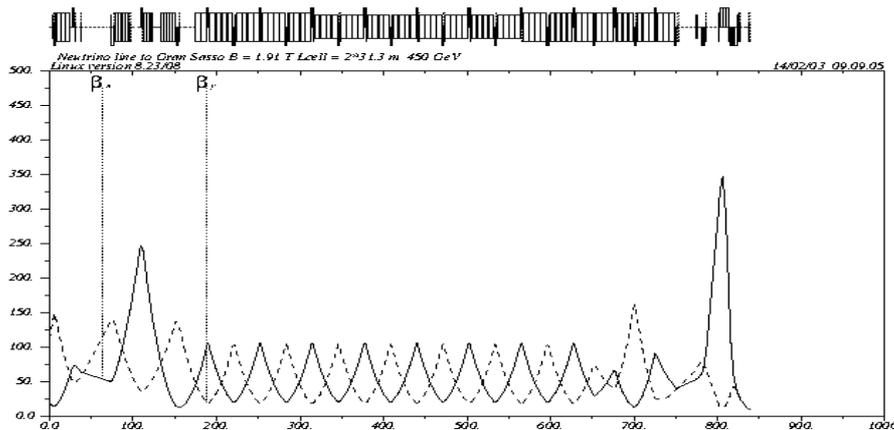
Figure 2. CNGS proton beam optics. Beta at focus in both planes = 10 m
