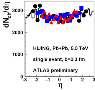
**Figure 1:** The generated (line) and reconstructed  $dN_{ch}/d\eta$  of a single central Pb+Pb event in the 1<sup>st</sup> (circles), 2<sup>nd</sup> (squares) and 3<sup>rd</sup> (triangles) layer of the Pixel detector.
