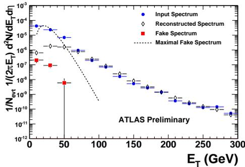
**Figure 4:** Input (filled circles) and reconstructed (diamonds) spectra for cone jets in central ( $dN_{ch}/d\eta = 2650$ ) Pb+Pb collisions. Squares and dashed line illustrate fake jet spectra with and without fake rejection cut applied.
