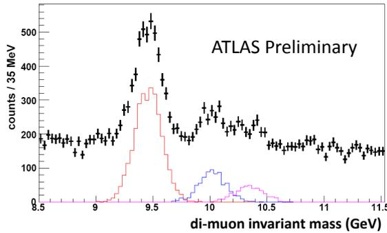
**Figure 6:** Di-muon invariant mass distribution as expected for one month of Pb+Pb running, taking into account acceptance, efficiency and background contribution, for decay muons in the barrel region only ( $|\eta| < 1$ ). Error bars show statistical errors only. Solid color histograms illustrate expected yields from  $\Upsilon$ ,  $\Upsilon'$  and  $\Upsilon''$  states, and points show the sum of signal and background.
