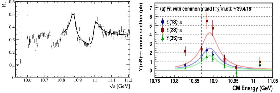
**Figure 3:** Left side:  $R_b$  measured by BABAR as a function of  $\sqrt{s}$  with the result of the fit superimposed. Right side: cross section for  $e^+e^- \rightarrow Y(NS)\pi^+\pi^-$ , ( $n = 1, 2, 3$ ) measured by Belle as a function of  $\sqrt{s}$  with the BW fit superimposed.
