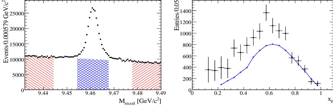
**Figure 2:** Left side: distribution of the recoil mass,  $M_{recoil}$ , for the selected  $\Upsilon(2S) \rightarrow \pi^+ \pi^- \Upsilon(1S)$  candidates. The cross hatching shows the signal region, and the lower and upper sideband regions are indicated by the diagonal shading. Right side: signal yield as a function of  $x_p$ . The dots represent the data and the solid line represents the expected contribution from the virtual photon process [13].
