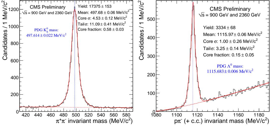
**Figure 3:** Left: Fitted  $\pi^+\pi^-$  mass spectrum for data. Right: Fitted  $p\pi^-$  (+ charge conjugate) mass spectrum for data. Uncertainties shown are statistical only.
