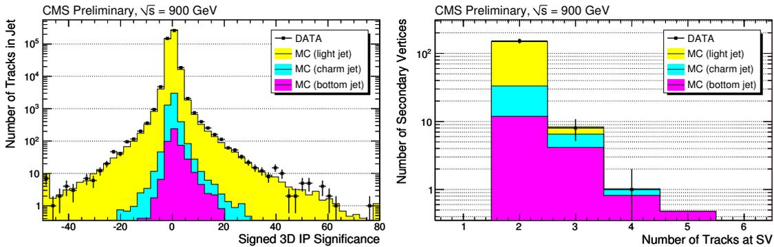
**Figure 5:** Left: Distribution of the significance of the three-dimensional impact parameter for all tracks in the jet. The data is shown as full circles while the simulated contributions from light flavor, charm and bottom are shown as filled histograms. Right: Number of tracks of the secondary vertex for vertices reconstructed inside jets.
