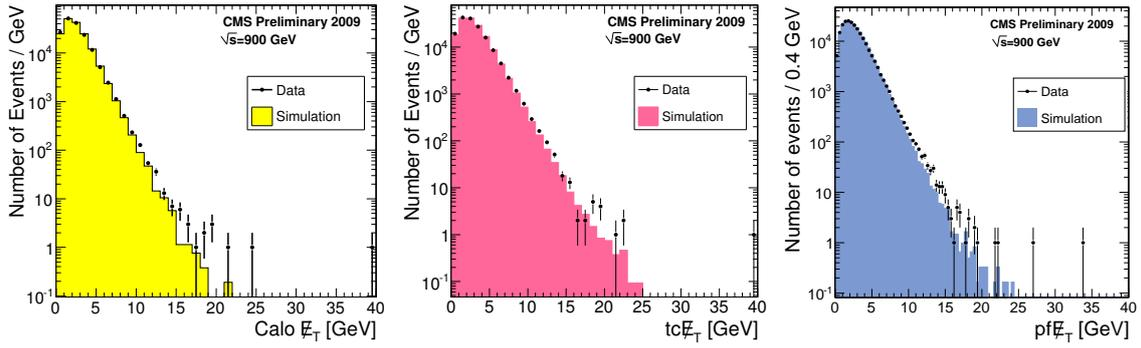
**Figure 8:** Comparisons of data and simulated missing  $E_T$  distributions at  $\sqrt{s} = 0.9$  TeV, for calorimeter, track corrected and particle flow, respectively.
