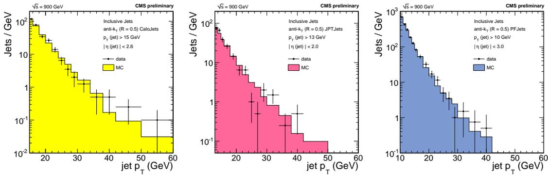
**Figure 7:** Comparisons of data and simulated inclusive jet  $p_T$  distributions at  $\sqrt{s} = 0.9$  TeV, for calorimeter, track corrected and particle flow jets, respectively.
