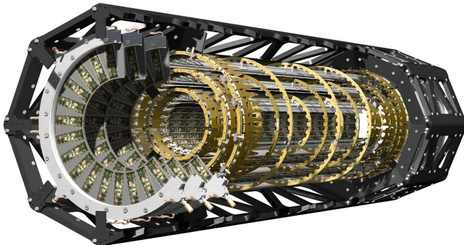
**Figure 1:** Schematic view of the ATLAS Pixel Detector.
