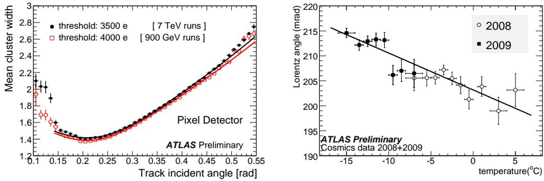
**Figure 7:** Lorentz angle measurements: (left) cluster size as function of the track incident angle for data at  $\sqrt{s} = 900$  GeV and 7 TeV, (right) value of  $\theta_L$  measured on cosmic-ray data as a function of the module temperature.
