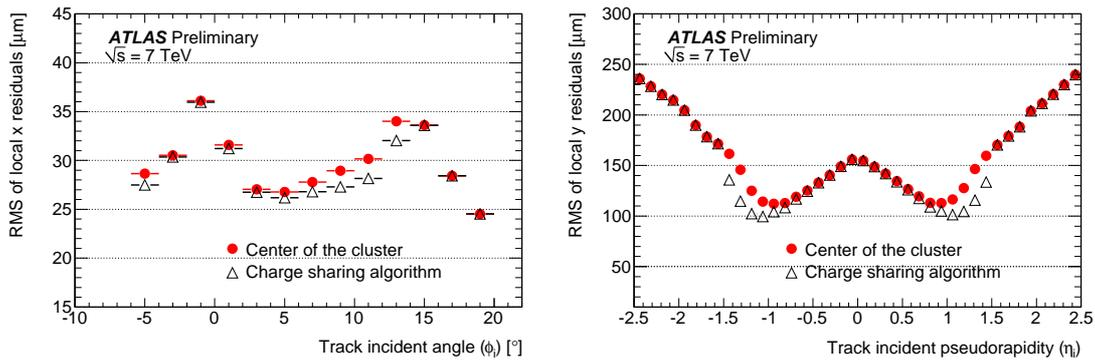
**Figure 6:** RMS of the residual distributions for cluster local- $x$  as a function of the track incident angle (left) and cluster local- $y$  as a function of track pseudorapidity (right).
