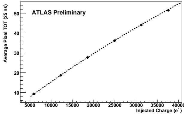
**Figure 3:** Average ToT value as a function of the collected charge for one FE chip. The dashed line is the curve used to calibrate the charge versus ToT relationship.
