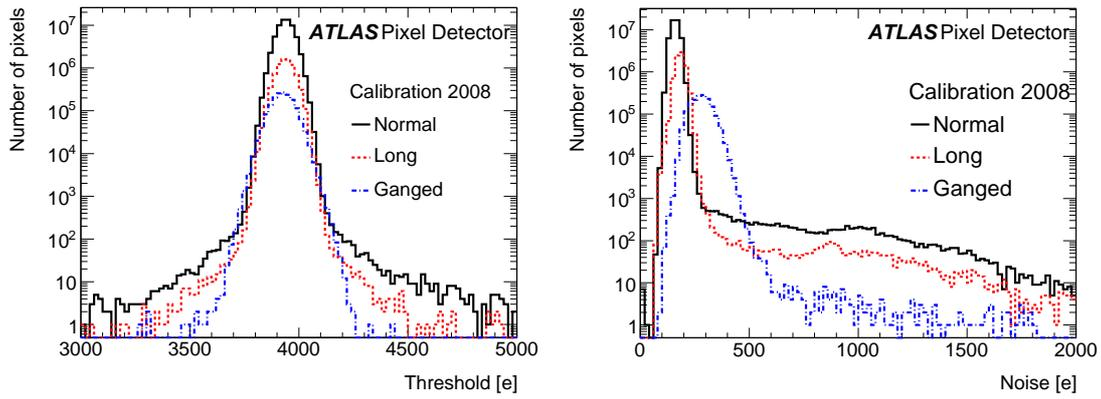
**Figure 2:** Pixel Detector threshold (left) and noise (right) distributions from calibrations based on charge injection.
