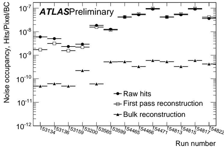
**Figure 4:** Pixel Detector noise rate from raw data, after the first pass of reconstruction (without offline noise masks) and after the bulk reconstruction using the offline noise mask.
