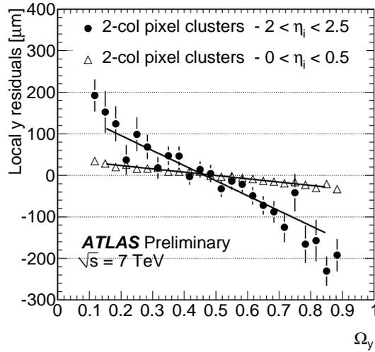
**Figure 5:** Pixel Detector residuals in the local- $y$  coordinate as a function of the charge sharing  $\Omega$  for 2-column clusters in different pseudorapidity regions.
