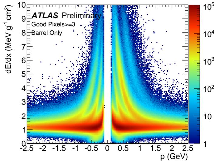
**Figure 8:**  $dE/dx$  measurement in the Pixel Detector as a function of  $Q \times p$  for particles with at least three associated hits.
