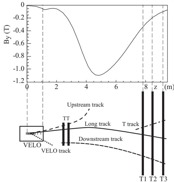
**Figure 1:** Vertical component of the LHCb dipole magnetic field (top) and different track types reconstructed by the tracking system (bottom). The total bending power of the magnet amounts to about 4 Tm.
