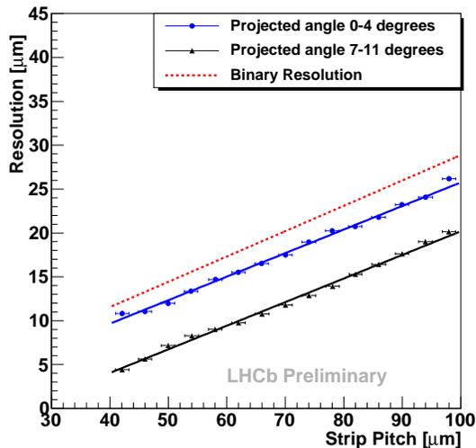
**Figure 3:** VELO hit resolution as function of strip pitch for different ranges of projected angle compared to binary resolution.
