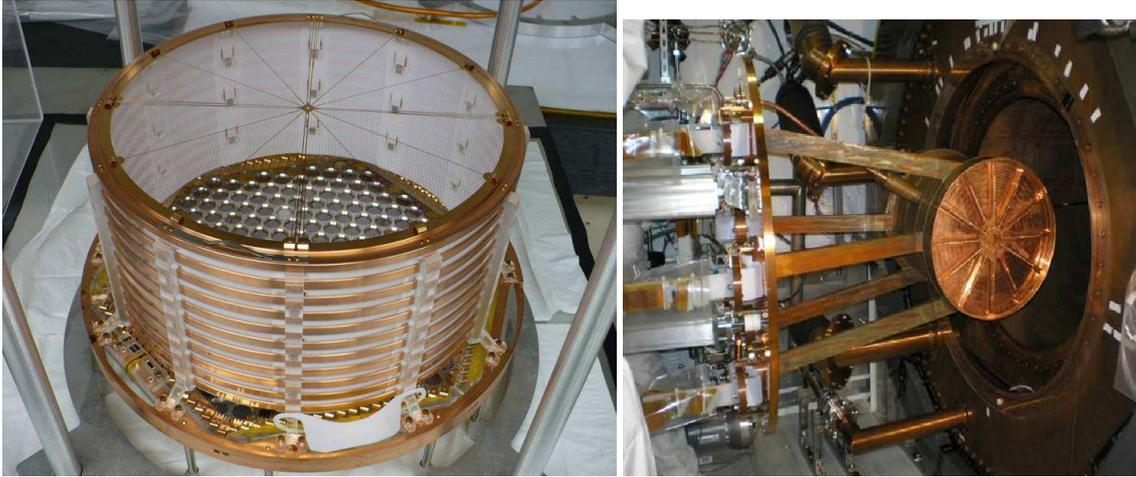
**Figure 1:** Left: One half of the EXO-200 TPC. Right: The fully instrumented liquid xenon vessel being inserted into the cryostat in January 2010.
