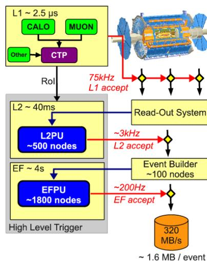
**Figure 1:** The ATLAS trigger with final design specifications for the rates, latencies and system sizes.
