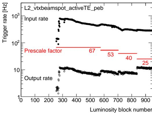
**Figure 2:** Here the L2\_vtxbeamspot\_activeTE\_peb chain (an arbitrary choice to illustrate the point) is initially disabled, then enabled at luminosity block (LB) 255 when LHC stable beams are declared. As the beam intensity falls, the input rate drops by almost a factor of 4. The prescale factor is reduced, without restarting the run, in a few steps to keep the output rate between about 6 to 12 Hz.
