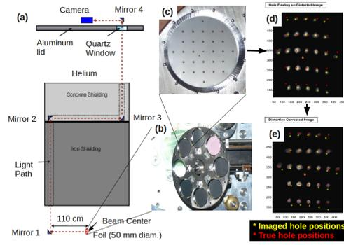
**Figure 2:** (a) Diagram of the OTR monitor optical system, where the beam direction is into the page. (b) Image of the OTR target wheel, including the installed targets. (c) Image of the calibration foil. (d) Backlit image of the calibration foil take by camera at the far end of the optical system. (e) Backlit image of the calibration foil after correction for the optical system distortions.
