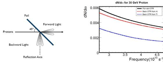
**Figure 1:** Left: Illustration of the transition radiation production at foil oriented  $45^\circ$  relative to the particle beam. Right: Spectrum of transition radiation production in the optical region.
