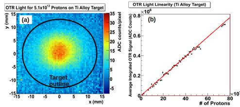
**Figure 3:** (a) Representative image of OTR light from a single beam pulse. (b) Linearity of OTR light production on the titanium foil as a function of protons per beam pulse.
