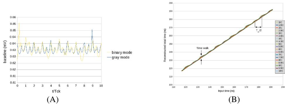
**Figure 2:** (A) Baseline modulation at the CFD output. (B) A Test Pulse delay scan was performed. The output times were reconstructed for charges from 1 fC to 10 fC. The spread of the curves represents the time-walk. Each hill corresponds to a clock transition, while the ideal curve would be a straight line
