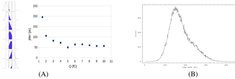
**Figure 1:** (A) Jitter measured from a matrix pixel. (B) The convolution with the NA62 Landau gives 92 ps
