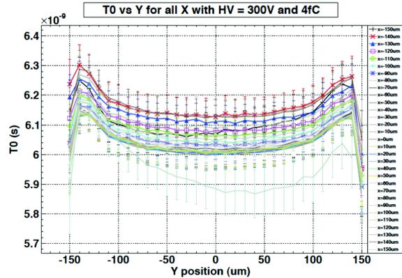
**Figure 4:** A complete laser scan of the pixel highlights the border effect contribution to timing error
