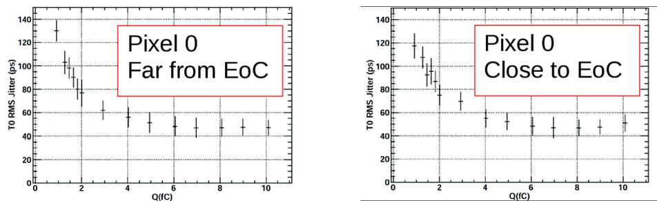
**Figure 3:** Time resolution measured for laser charge injection at the pixel center results in 70 ps at 2.4 fC
