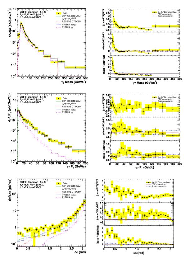
**Figure 1:** The measured differential cross sections compared with three theoretical predictions discussed in the text. **Left:** absolute comparisons. **Right:** fractional deviations of the data from the predictions. Fractional deviations for PYTHIA refer to the  $\gamma\gamma + \gamma j$  calculation.
