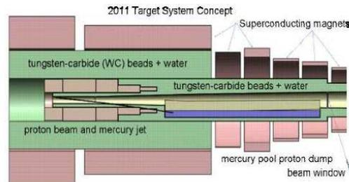
**Figure 2:** Neutrino Factory target.
