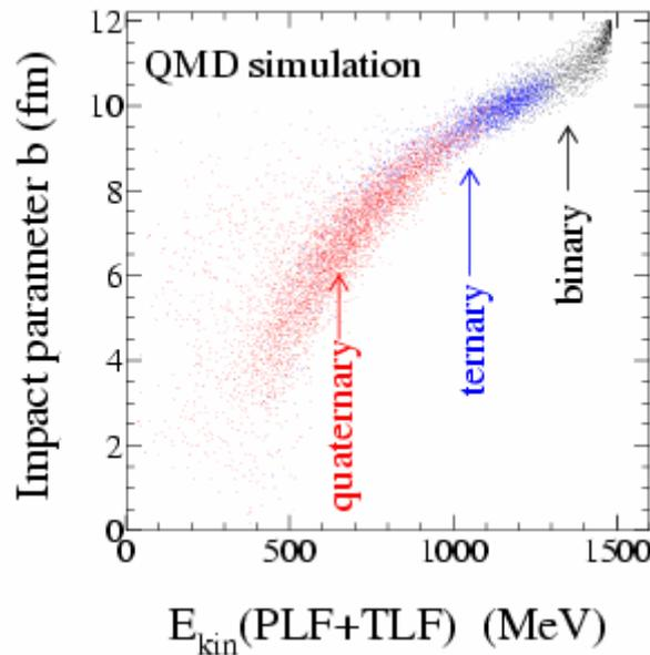
**Fig. 2** Correlation between the total kinetic energy and impact parameter for binary, ternary and quaternary reactions in  $^{197}\text{Au} + ^{197}\text{Au}$  collisions at 15 MeV/nucleon, simulated with the QMD model of Łukasik [4]. Points representing binary, ternary and quaternary events are marked with different colors: black, blue and pink, respectively. This correlation can be used to calibrate the observed inelasticity of the reaction as a measure of the impact parameter.
