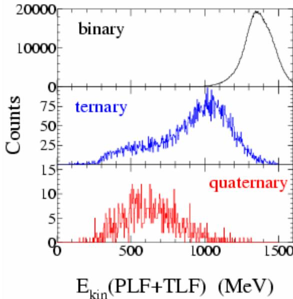
**Fig. 1** Total kinetic energy spectra of fragments for binary (top), ternary (middle) and quaternary (bottom) reactions. For ternary and quaternary reactions  $E_{\text{kin}}(\text{PLF}+\text{TLF})$  is determined as the kinetic energy of the *primary* PLF+TLF system. The velocity vector of PLF
