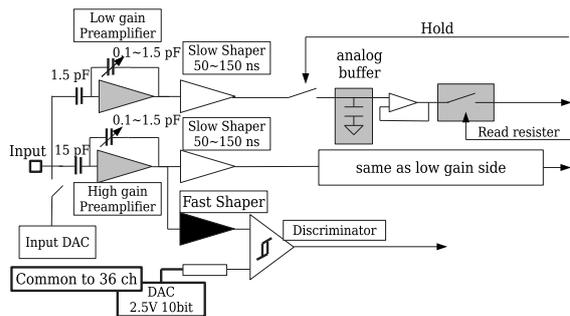
**Figure 2:** The Schematic of one channel in EASIROC.
