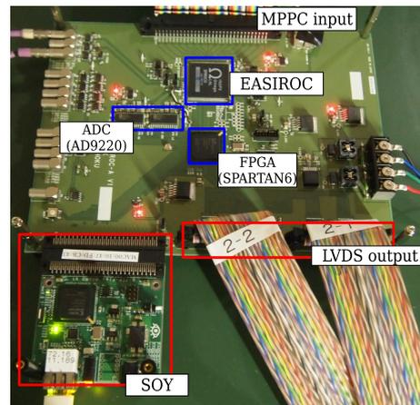
**Figure 3:** Picture of the evaluation board.
