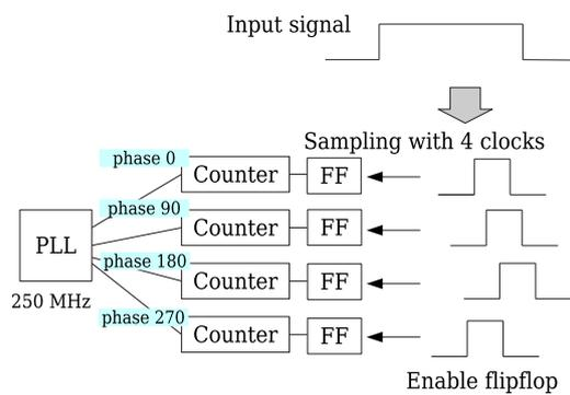
**Figure 6:** The schematic of MHTDC in FPGA.
