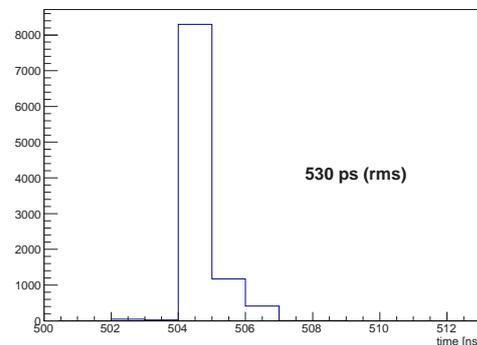
**Figure 7:** The distribution of MHTDC obtained by injecting a charge.
