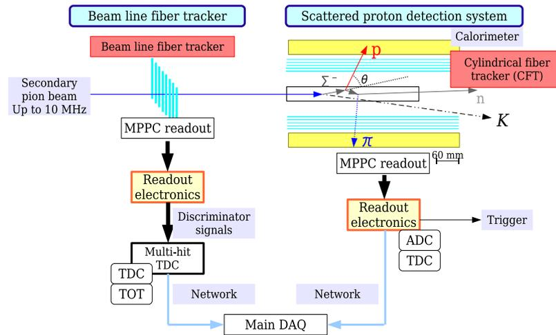
Figure 1: Experimental setup of J-PARC E40.
