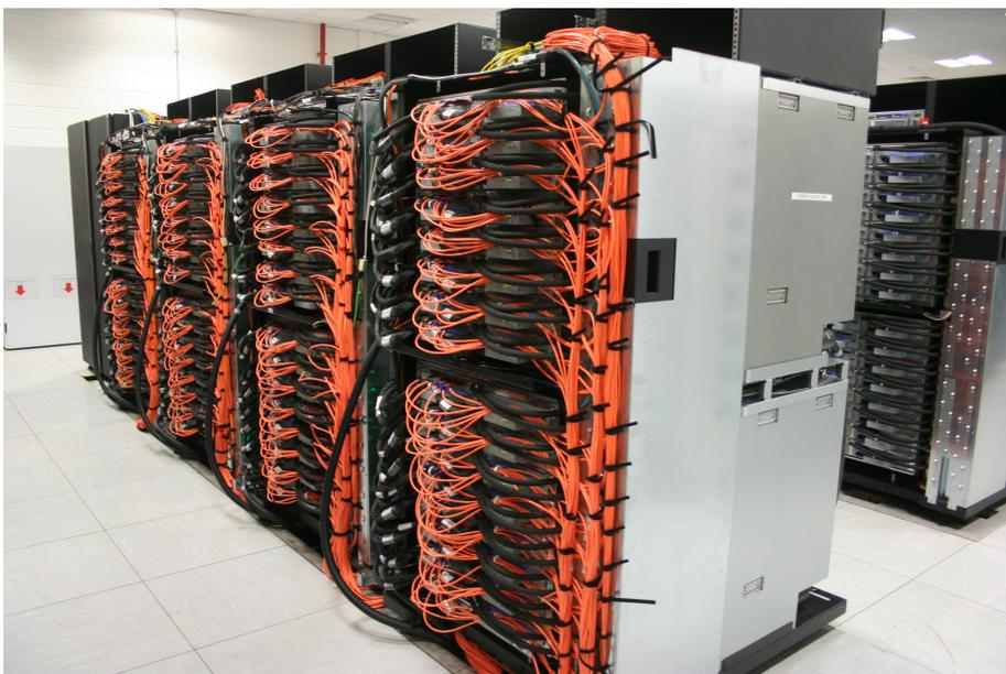
**Figure 2:** The 1.26Pflop/s Edinburgh BlueGene/Q DiRAC system, comprising six racks.
