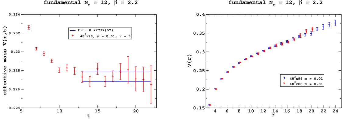
**Figure 1:** (left) The effective mass  $V(r,t)$  and the fitted potential  $V(r)$  for the  $N_f = 12$  fundamental model at  $r = 5$  on a  $48^3 \times 96$  volume at fermion mass  $ma = 0.01$ . The quality of the correlated fit is  $\chi^2/N_{\text{dof}} = 2.0$ . (right) Volume dependence of the potential  $V(r)$  with lattice volumes  $48^3 \times 96$  and  $40^3 \times 80$  at mass  $ma = 0.01$ .
