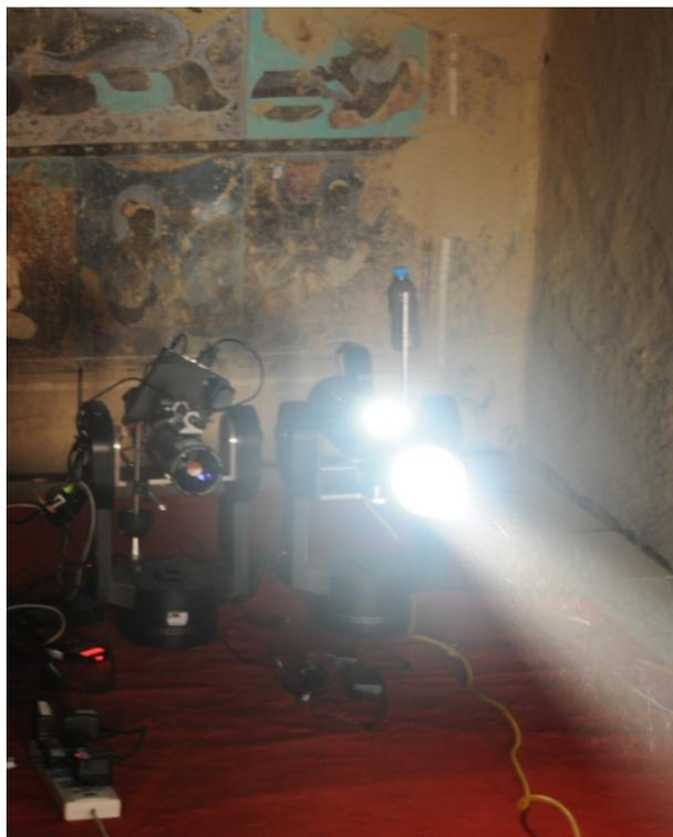
**Figure 3:** The spectral imaging system PRISMS in cave 465 of Mogao caves, Dunhuang. The imaging system is on the left of the lighting system.
