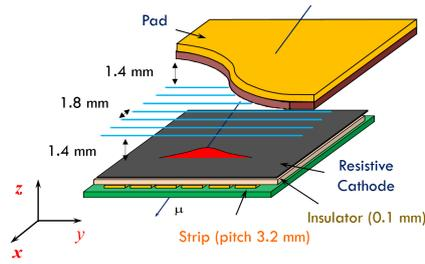
**Figure 1:** The structure of the proposed sTGC detector.
