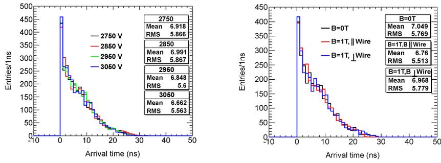
**Figure 2:** Earliest cluster arrival time distributions for different high voltages (left) and under B field (right).
