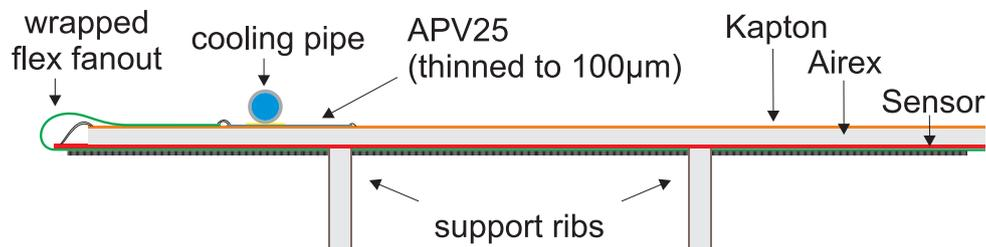
**Figure 6:** Chip-on-Sensor concept with wrapped flex fanout around the sensor edge.
