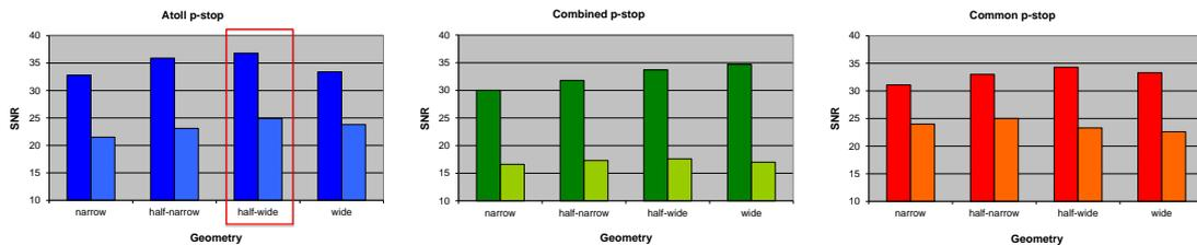
**Figure 4:** Signal to noise ratios of the three different p-stop layouts. The left bars (dark colors) show the unirradiated case while the right bars (bright colors) show the irradiated figures. The geometry which performed best is marked with a red box.
