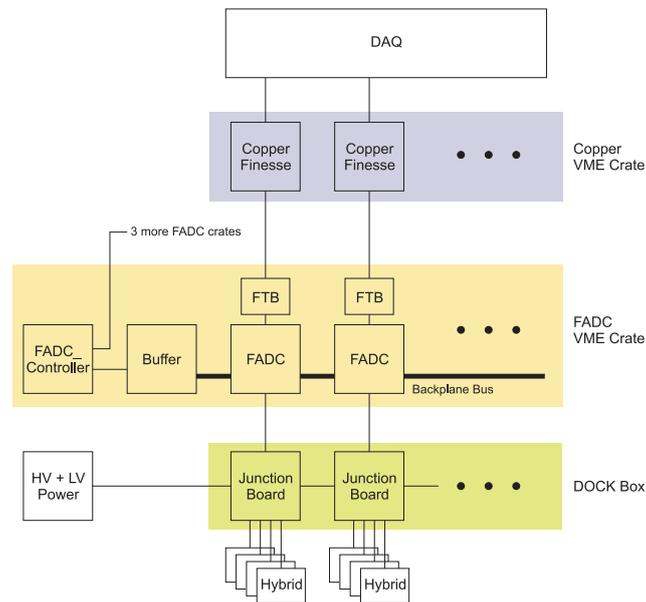
**Figure 5:** DAQ chain. The DOCK boxes are located inside the Belle II experiment (but outside of the SVD), the FADC VME crates are located on top of the experiment in dedicated racks, while the interface to the central DAQ of Belle II (called COPPER) is housed in the electronics hut next to the experiment.
