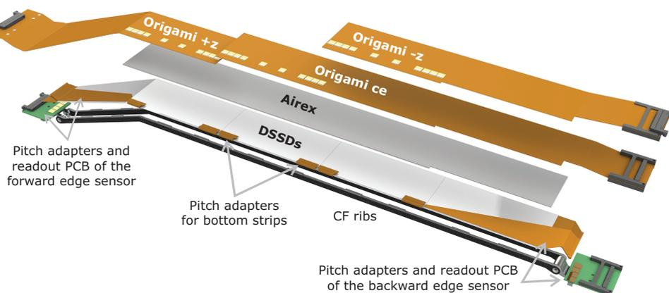
**Figure 7:** Exploded view of one ladder of outermost layer 6.
