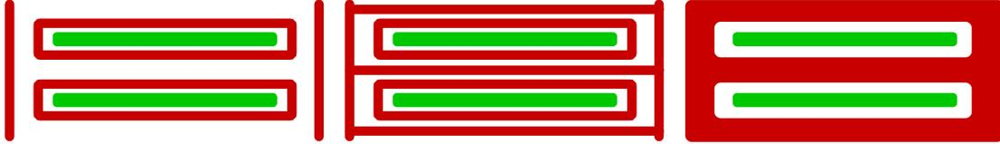
**Figure 3:** Schematic layout of atoll (left), combined (center) and common (right) p-stop layout. P-type implantation is shown in red, n-type implantation in green.
