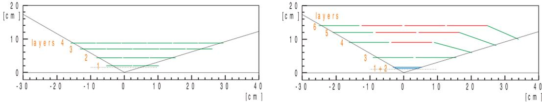
**Figure 2:** Layout of the layers of the Belle (left) and Belle II SVD (right). In the latter case, layers 1 and 2 (shown in blue) are an additional sub-detector of Belle II called PXD which is made of DEPFET pixel detectors. Layers 4-6 comprise double sided silicon strip detectors (DSSDs). Each red line corresponds to a so-called Origami module with readout electronics inside the active volume, while the green lines show modules read out by hybrids outside the acceptance region.
