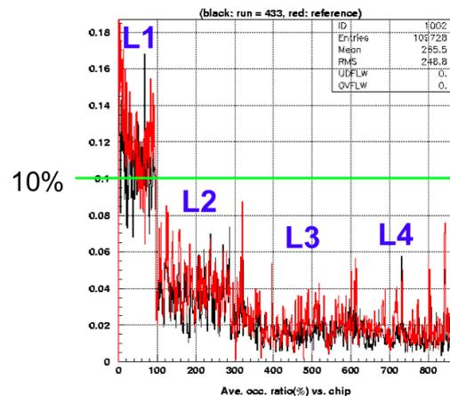
**Figure 1:** Occupancy during a typical run of Belle at maximum luminosity. The innermost layer L1 observed occupancies of up to 18%, which is above the limit of 10%.
