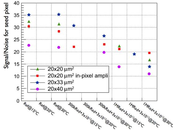
**Figure 2:** Signal over noise ratio evolution of different MIMOSA-32 pixel designs with the ionising and non-ionising radiation loads and different air-cooling temperatures.
