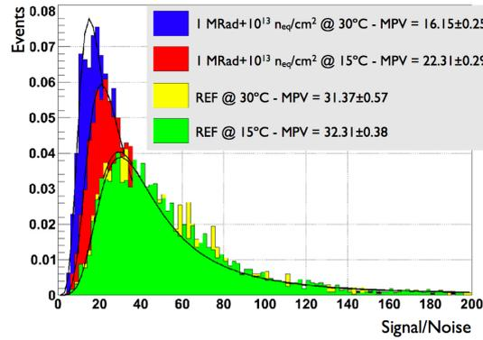
**Figure 1:** Observed response of MIMOSA-32 ( $20 \times 20 \mu m^2$  pixels) to  $\sim 100$  GeV pions. The figure shows the signal over noise ratio (SNR) distribution before irradiation and after a combined load of 1 MRad and  $10^{13}$   $n_{eq}/cm^2$  at different air-cooling temperatures.
