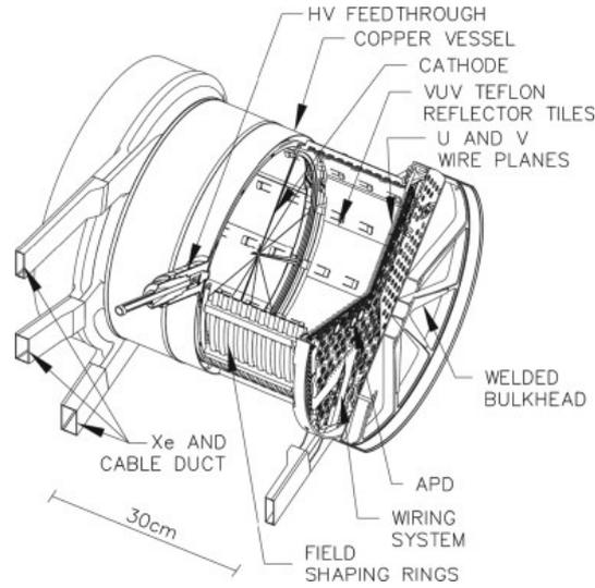
**Figure 1:** Cutaway view of the EXO-200 TPC.
