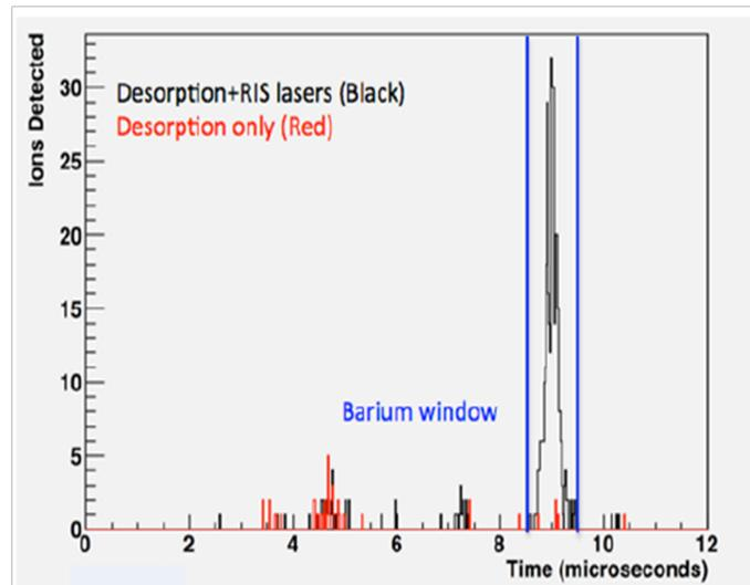
**Figure 5:** TOF spectrum for desorped ions from a silicon surface with a thin layer of Ba.
