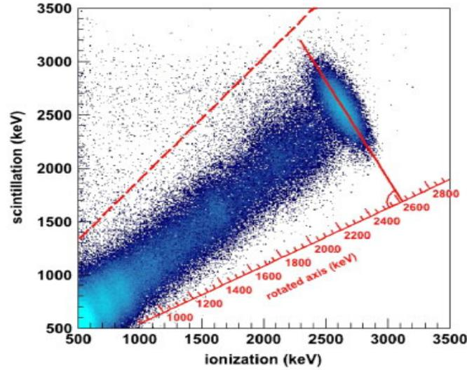
**Figure 2:** Anti-correlation between ionization and scintillation for SS events from  $^{228}\text{Th}$  source.
