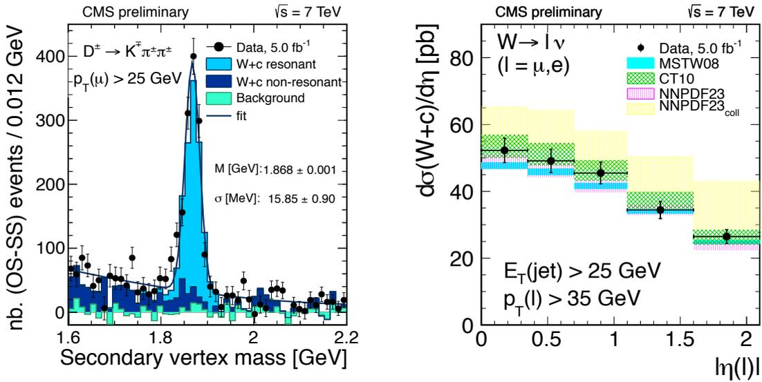
**Figure 3:** Left: the reconstructed secondary vertex mass of the  $D^\pm \rightarrow K^\mp \pi^\pm \pi^\pm$  decay in the W+c final state, after correcting the predicted branching ratio and subtracting the backgrounds. Right: the differential W+c cross section measurement as a function of  $|\eta(l)|$  compared with the predictions from different PDFs.
