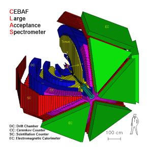
**Figure 3:** Schematic diagram of CLAS. Four of the six CLAS sectors are displayed, with their different detector layers.
