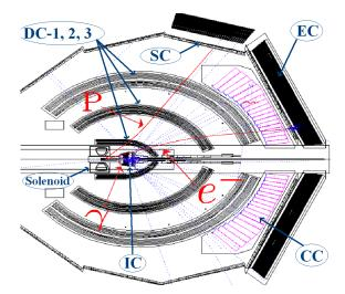
**Figure 4:** A typical  $ep\gamma$  event in a side view of CLAS. The solenoid and the Inner Calorimeter, which are not part of the standard CLAS equipment, can be seen in the central part.
