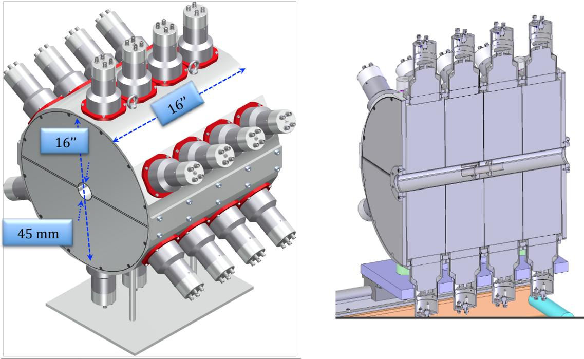
**Figure 2:** Mechanical design of the Summing NaI detector (SuN). SuN consists of eight optically-isolated segments, each being read by three PMTs. The figure on the right-hand side shows a cut-view of SuN where the target location and the detector segmentation are visible.
