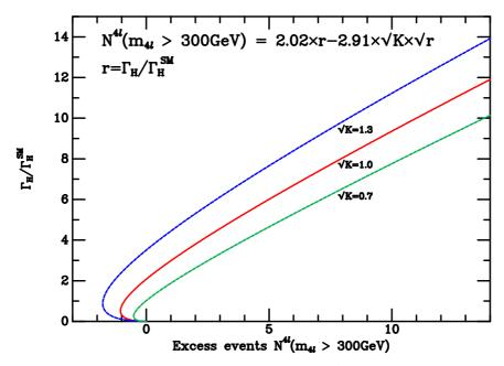
**Figure 6:** Influence of relative K-factor on extracted limit for  $\Gamma_H/\Gamma_H^{SM}$  as a function of the number of excess events from gg-induced Higgs boson related processes.
