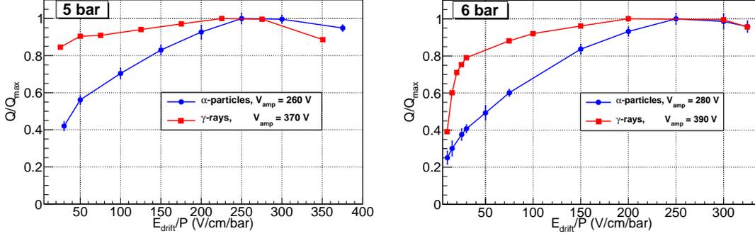
**Figure 3:** Fraction of charge collected for  $\alpha$ -particles and  $\gamma$ -rays with  $E_d/P$  at 5 bar (left) and 6 bar (right).
