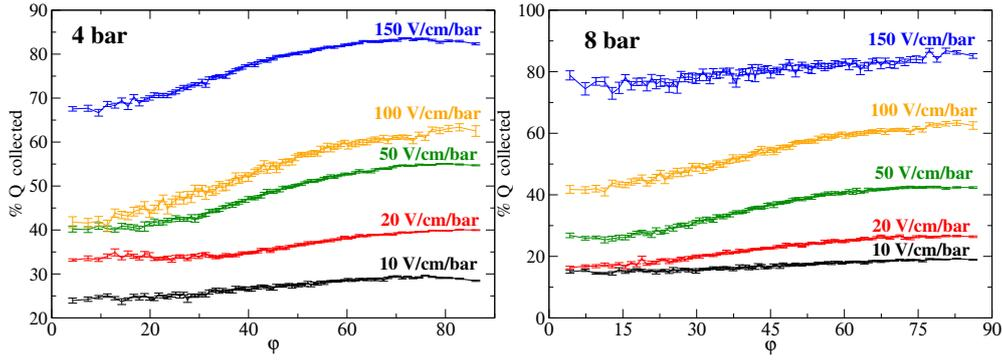
**Figure 5:** Dependence of the percentage of charge collected on the track angle ( $\phi$ ) at 4 bar (left) and 8 bar (right). This is a profile plot obtained from the scatter-plot of the charge vs track angle, in which the percentage of charge is obtained as the ratio of the mean charge for each angle bin to the maximum charge for each drift field.
