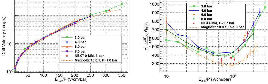
**Figure 4:** Drift velocity (left) and longitudinal diffusion coefficient (divided by  $\sqrt{P}$ ),  $D_L^*$ , (right) as a function of  $E_d/P$ , for pressures between 3 and 8 bar in a mixture of 2.2%TMA together with Magboltz calculations [7] and previous experimental results taken with the same mixture [2, 6].
