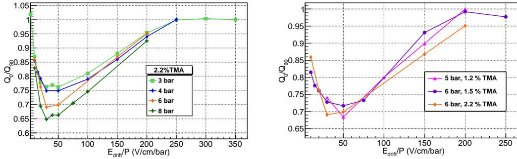
**Figure 6:** Ratio between charge collected for tracks parallel and perpendicular to the electric field ( $Q_0/Q_{90}$ ) as a function of the reduced field ( $E_d/P$ ). Left: Results for different pressures (3 to 8 bar) in a mixture of Xe+2.2%TMA, Right: Results for different Xe+TMA admixtures (1.2-2.2%TMA).
