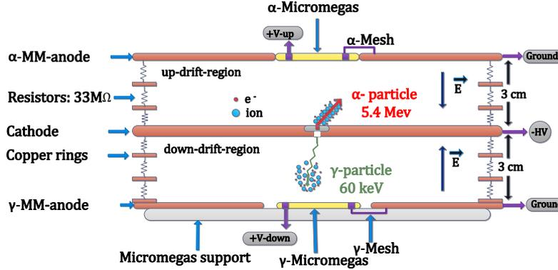
**Figure 1:** Schematic representation of the drift field configuration used to study the electron-ion recombination. The microbulk-Micromegas readouts and the voltage configuration are also shown.
