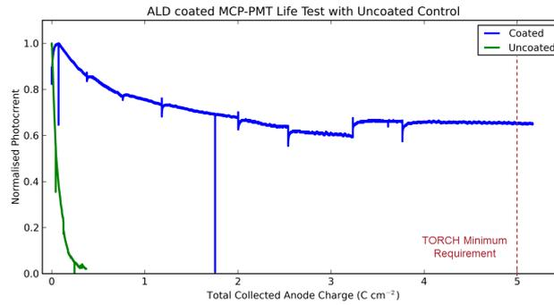
**Figure 5:** Initial measurement of gain as a function of integrated anode charge. After an initial decrease, the photocathode response is shown to be stable and fully satisfying TORCH requirements. The uncoated MCP-PMT is seen to degrade after  $\mathcal{O}(100 \text{ mC/cm}^2)$  [8]
