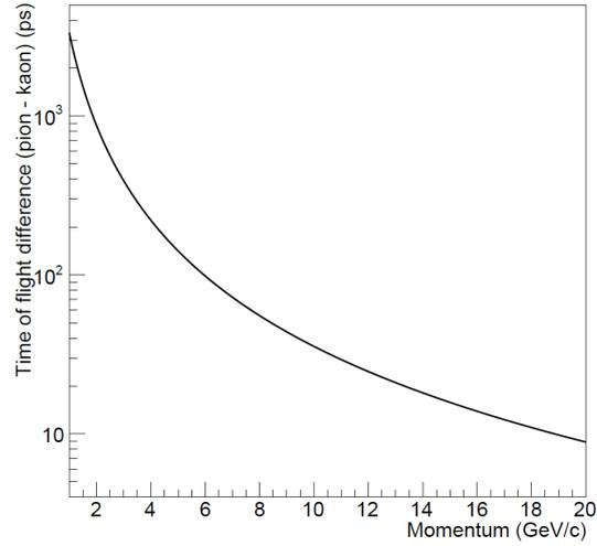
**Figure 2:** The time-of-flight difference between pions and kaons as a function of momentum over a flight distance of 9.5m.
