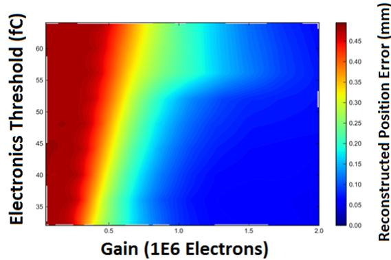
**Figure 7:** The uncertainty in reconstructed photon position with charge sharing. The electronics threshold should be a minimum of 50 fC to reach the required timing resolution [13].
