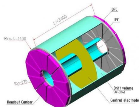
**Figure 3:** Layout of the TPC detector.
