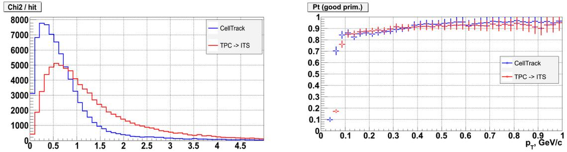
**Figure 14:** Left - distribution of  $\chi^2 / \text{hit}$ ; right - primary track finding efficiency vs  $p_T$ . Here “CellTrack” are the tracks found by the CA algorithm and fitted by the Kalman filter. “TPC  $\rightarrow$  ITS” - tracks were found in TPC using the Kalman filter and extrapolated to ITS.
