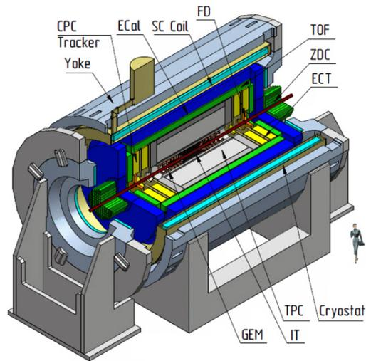
**Figure 1:** General view of the MPD detector. The detector includes the following subsystems: superconductor solenoid (SC Coil) and magnet yoke, time-projection chamber (TPC), inner tracking system (IT), time-of-flight counters (TOF), electromagnetic calorimeter (EMC), straw-tube endcap tracker (ECT), cathode pad chambers (CPC), gas electron multiplier detectors (GEM), fast forward detectors (FD) and zero degree calorimeter (ZDC).
