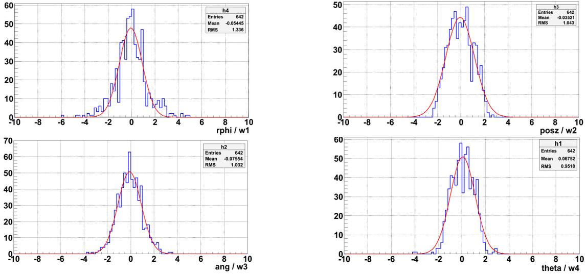
**Figure 12:** Distributions of pulls. Here  $rphi, posz, ang, theta$  are the true errors,  $w1, w2, w3, w4$  are the calculated ones.
