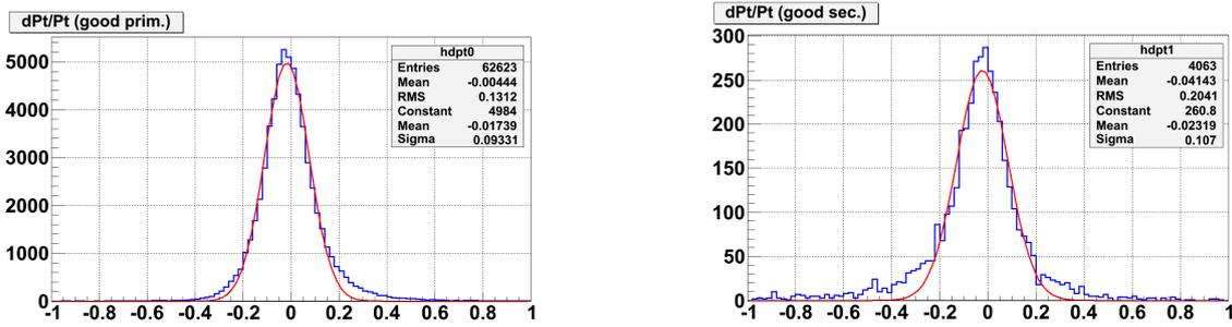
**Figure 13:** Left - the relative momentum resolution for primary tracks; right - the relative momentum resolution for secondary tracks.
