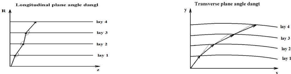
**Figure 8:** Left - schematic representation of the angle  $dangl$  in the longitudinal plane; right - schematic representation of the angle  $dangt$  in the transverse plane.
