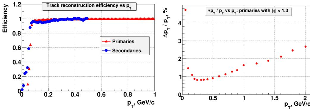
**Figure 6:** Left – track reconstruction efficiency as a function of track transverse momentum  $p_T$  for primary and secondary particles; right – relative transverse momentum resolution for primary tracks with pseudorapidity  $|\eta| < 1.3$  reconstructed in TPC.
