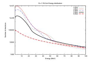
Fig. 7: Electron energy spectra at different altitudes in an electric field of -1.7 kV/cm
