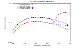
**Fig. 1:** Number of electrons and positrons as a function of atmospheric depth in an electric field of 1.7 kV/cm. (electric field area: 457-599 g/cm<sup>2</sup>)
