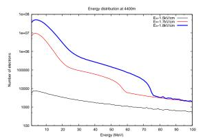
**Fig. 5:** Energy distribution of electrons and positrons in electric field of -1.7 kV/cm and the same in absence of a field at the altitude of 4400 m
