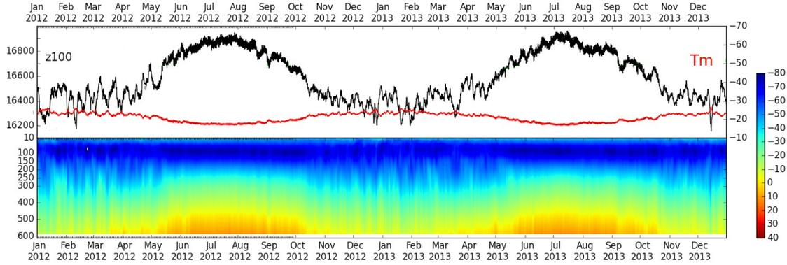
**Fig. 4.** Upper panel: the high of the level of muon generation  $Z_{100}$ , m (left axis, black line) and the mass-average temperature (right axis, red line). Bottom panel: temperature altitude distribution in the atmosphere by the isobaric levels for the YangBaJing muon telescope 2012-2013.
