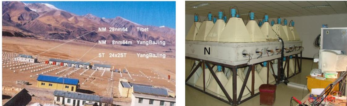
**Fig. 1.** The YangBaJing multidirectional muon telescope.
