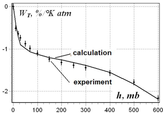
Fig. 7. Altitude dependence of the estimated (continuous) and experimental densities of the temperature coefficient on ambient pressure.
