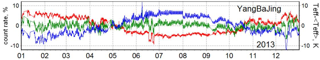
**Fig. 5.** Variations of the effective temperature  $T_{\text{eff}}$  (blue line), count rate variations (vertical) of the YangBaJing muon telescope - uncorrected (red line) and corrected (green line) for the temperature effect for 2012-2013.
