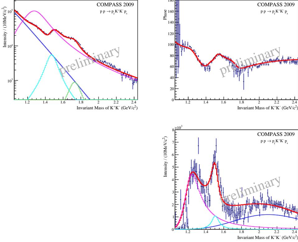
**Figure 6:** Mass-dependent parametrisation (red curve) of  $S_0$ -wave (top left) and  $D_0$ -wave (bottom right) intensities and their relative phase (top right) for the centrally produced  $K^+K^-$  system. The non-resonant (blue) and Breit-Wigner (other colours, see text) contributions to the intensity spectra are indicated.
