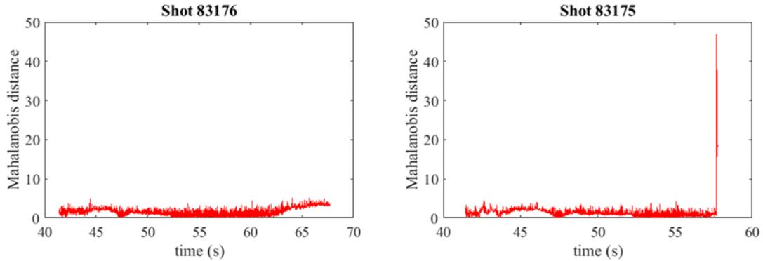
Fig. 3: Temporal evolution of the Mahalanobis distance in safe and disruptive discharges. The large increase at the end of discharge 83175 identifies outliers.
