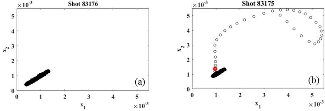
Fig. 1: Scatterplots with same scales for a non-disruptive discharge and a disruptive one. The data dispersion is much larger close to a disruption. (a) Compact cluster. (b) The presence of outliers is related to a forthcoming disruption.
