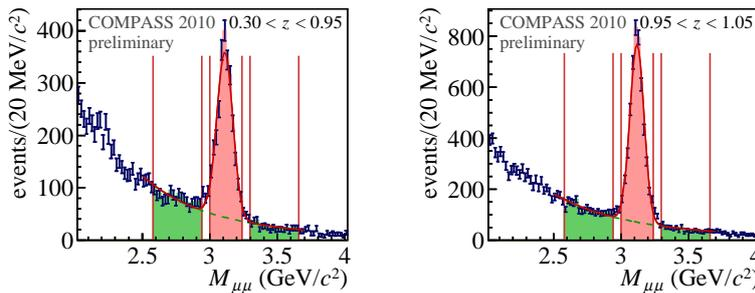
Figure 1: Dimuon invariant mass in the two  $z$ -intervals. Left: inclusive events, right: exclusive events. The boundaries of the side-bands and the signal band are denoted by vertical red lines. The red fit to the data is the normal distribution plus background in the form  $AN(M_{\mu\mu}, \mu, \sigma) + BM_{\mu\mu}^C$ . The dotted green line is the background estimation  $BM_{\mu\mu}^C$ .
