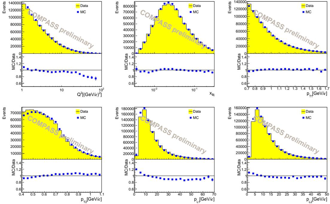
Figure 3: Comparison of kinematic variables distributions from experimental and MC2010 high- $p_T$  proton data, respectively.
