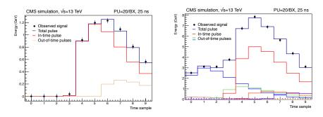
**Figure 1:** Examples of fitted ECAL pulses for signals in EB (left) and EE (right) with 20 pileup interactions. Dots represent the 10 digitized samples and the red distributions (other light colors) represent the fitted intime (out-of-time) pulses. The dark blue histograms represent the sum of all the fitted contributions.
