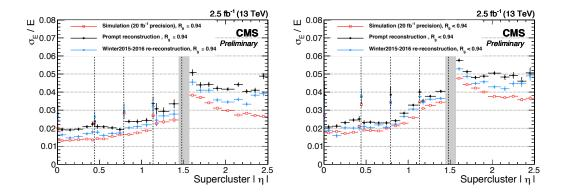
**Figure 3:** Relative electron energy resolution unfolded in bins of pseudo rapidity for the barrel and the endcaps using electrons from  $Z \rightarrow ee$  decays. The resolution is shown for low (left) and high (right) bremsstrahlung electrons ( $R_9 > 0.94$  and  $R_9 < 0.94$  respectively, with  $R_9 = E_{3x3}/E_{\text{Supercluster}}$ ).
