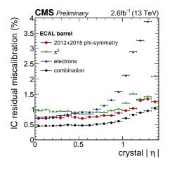
**Figure 2:** Precisions of the EB inter-calibration methods, as a function of pseudo rapidity, for the dataset recorded during 2015.
