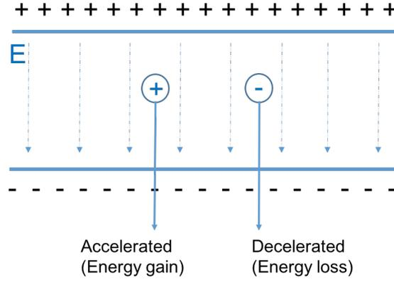
Figure 2: Charged particle motion in electric field
