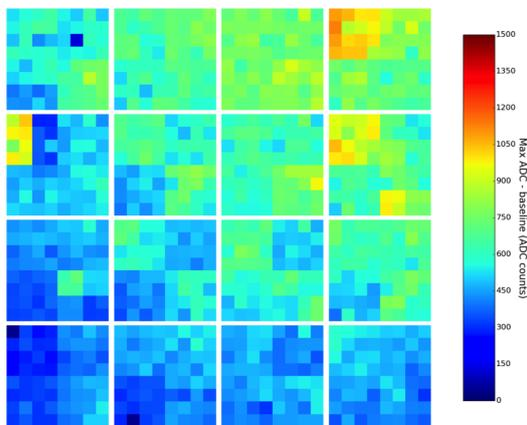
Figure 7: Uncalibrated image of a light flash recorded with the prototype camera in the laboratory
