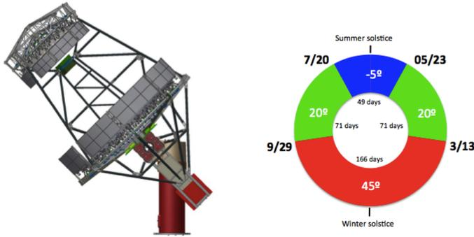
Figure 1: pSCT Parking concept. Three parking positions at elevations  $-5^\circ$ ,  $20^\circ$  and  $45^\circ$  will be used during the year.
