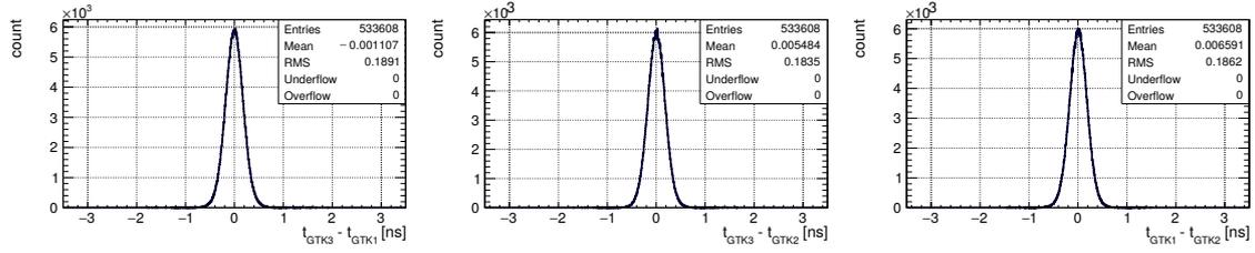
**Figure 6:** Time differences of pixel hits recorded in the three GigaTracker stations in fully reconstructed  $K^+ \rightarrow \pi^+ \pi^+ \pi^-$  decays (2016 data). The RMS of the three distributions are:  $RMS(t_{GTK1} - t_{GTK3})=189$  ps,  $RMS(t_{GTK2} - t_{GTK3})=184$  ps and  $RMS(t_{GTK1} - t_{GTK2})=186$  ps. These values are only few ps larger than the standard deviations from a gaussian fit thus indicating the small contribution of non-gaussian tails.
