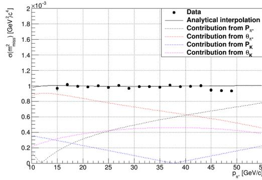
**Figure 8:** Gaussian resolution of the  $m_{miss}^2$  measured on a  $K^+ \rightarrow \pi^+ \pi^0$  sample as a function of charged pion momentum (2016 data). The black solid line is an analytical interpolation using the expected resolutions for GigaTracker and STRAW. The dashed lines correspond to the contributions of the individual quantities entering in the computation of  $m_{miss}^2$ .
