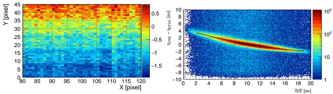
**Figure 4:** GigaTracker hit time corrections used in offline reconstruction. Left: time offsets in ns of the individual pixels in a TDCPix chip. Right: time-walk as a function of the signal height measured by the time-over-threshold (ToT). The line corresponds to the result of a quadratic fit of the most probable value of the time-walk.
