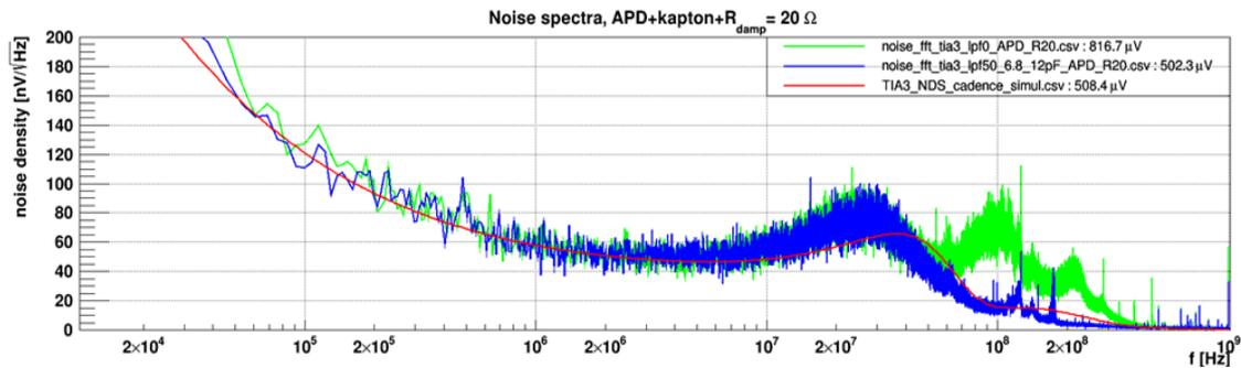
Figure 4: Noise spectral density of CATIA connected to APDs as in ECAL. In green without bandwidth limitations, in blue with a low pass filter at 50 MHz<sup>1</sup> and in red the simulation results (<sup>1</sup> optimal TIA output filter frequency to limit the TIA noise bandwidth).
