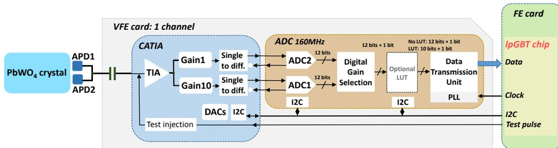
**Figure 1:** New VFE electronics is formed with CATIA ASIC [Trans-Impedance Amplifier (TIA) with two gain ranges (1 and 10) and 50 MHz of bandwidth (RC of 3 ns)] and 12-bit ADC [two channels sampling each at 160 MSPS].
