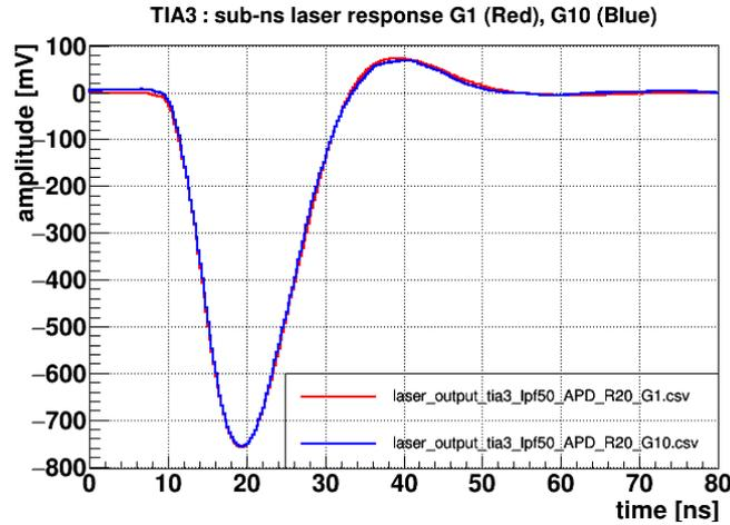
Figure 3: Signals measured at the output of Gain1 and Gain10 stages.
