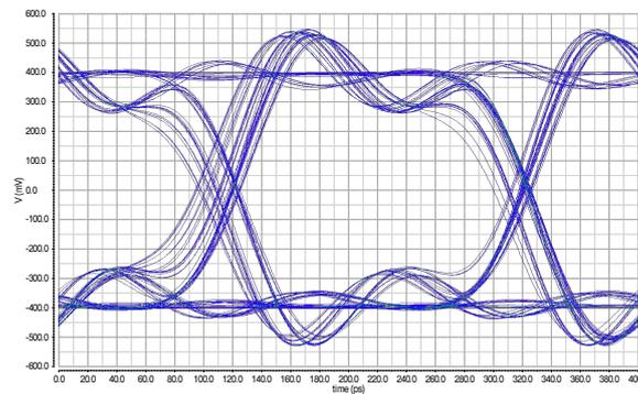
**Figure 3:** Eye diagram of the simulated response of the LAPA pseudo-LVDS driver integrated in a channel of the test chip. The input is a 2.5 GHz differential signal of 400 mV, with 50 ps of rising/falling time,  $V_{CM}$  of 0.8 V. The simulated peak to peak jitter is 45 ps.
