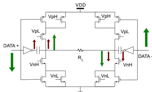
**Figure 2:** Schema of the pre-emphasis. An inverting stage driven by the same data that drives the main driver is directly capacitively coupled to out pads. The effect of the pre-emphasis on the output is represented in red.
