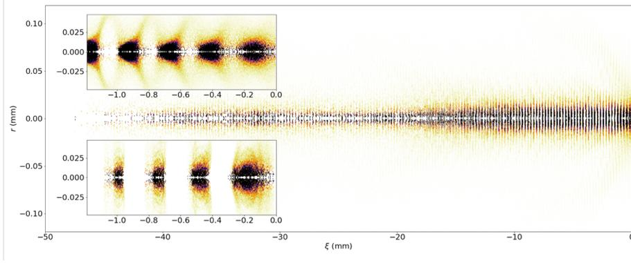
**Figure 1:** Example beam profile for a proton drive beam as it undergoes self-modulation. The beam parameters correspond to the "matched to ellipse" beam outlined in Table 1 at propagation distance of  $z = 0.4$  m. Inset, top left: beam profile zoomed in on the first few microbunches at  $z = 0.4$  m. Inset, bottom left: beam profile zoomed in on the first few microbunches at  $z = 2$  m, after saturation has occurred.
