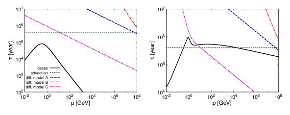
**Figure 1:** Energy dependence of the characteristic timescales (expressed in years) of cosmic ray electrons (left panel) and protons (right panel) for the parameters of Tab. 1. Black thick lines represent energy losses, green dotted lines show the advection timescales. The timescales of diffusion are represented by blue dashed lines in the case of Model A, red dot-dashed in the case of Model B and magenta dot-dot-dashed in the Model C.
