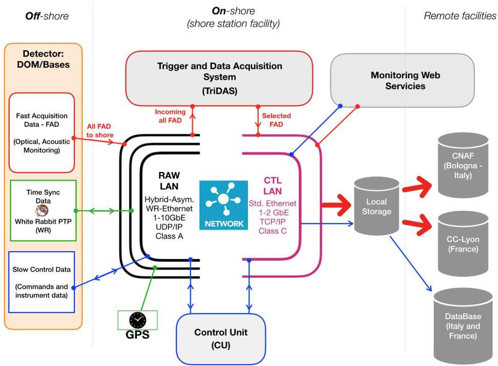
Figure 2: Outline of KM3NeT DAQ components.
