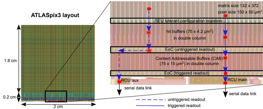
Figure 1: ATLASp3 top layout showing triggered and triggerless readout data path
