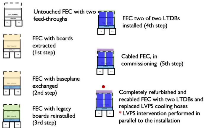
**Figure 2:** Schematics showing installation status for each of the calorimeter crates in the barrel and endcap regions for sides A and C. The colors of the crates in the schematics are described in the legend below, which also details the order of steps involved in the refurbishment process.
