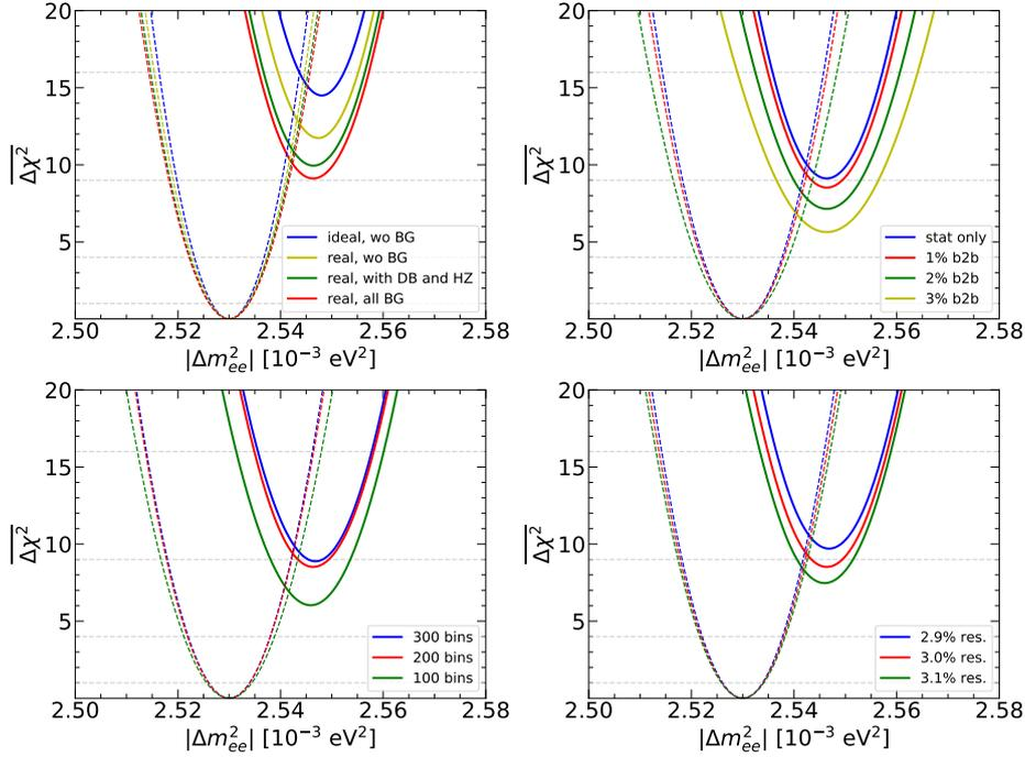
**Figure 1:** The effects of the real reactor core-detector baseline distribution as well as of the two types of backgrounds: from the distant reactors Daya Bay (DB) and Huizhou (HZ) as well as from other sources (accidental, cosmogenic, etc.). Also shown are the effects of varying the number of bins, the energy resolution and the flux shape uncertainty.
