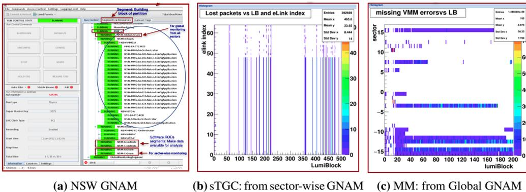
**Figure 3:** An example of a sTGC (b) and MM (c) histogram produced by NSW GNAM (a).
